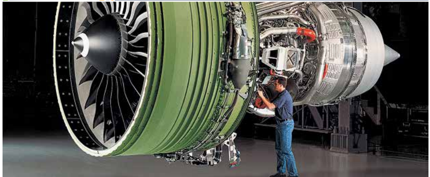
GE aviation engineer installs 3-D printed aircraft components on the GE90 turbofan jet engine.
